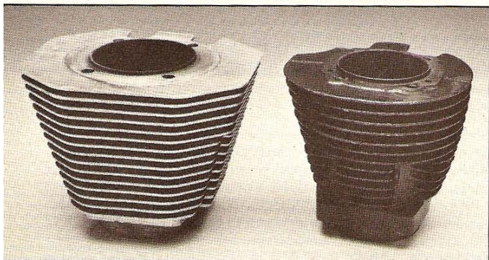
Even with larger bore, replacement barrel (left) is nearly 4 lb. lighter than stock. Aluminum is cast around manganese iron liner.
