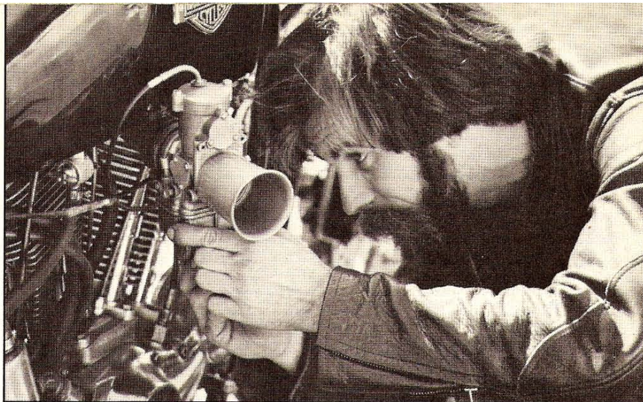
Breese performs last-minute jetting change on highly-accessible Dell'Ortos. Accelerator pumps are removed "for good gas mileage."
