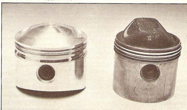
Engine uses 0.42-over S&S pistons (left) and a 9:1 compression ratio. At right is stock Sportster piston.
