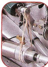
Below: Left-hand view of chassis and engine shows two (lower) air cylinders that operate the shifting linkage. Upper cylinder raises and lowers rear wheel. With wheel in upper position, the Breese liner can be rested on its fairing, thus eliminating the troublesome skids seen on all previous two-wheeled streamliners. Rubber bands on upper cylinder remove play and damp rattle.
