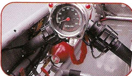
Right: A tachometer is the sole instrument—at high speeds there is little time to glance at more. Various switches dispatch parachutes, raise and lower the rear wheel, operate the fire extinguisher and kill the ignition.
